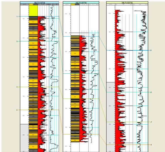
Fig. 5: Lithologic correlation along the three wells
